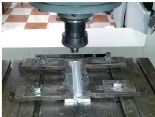
Figure 4 Used fixture to clamp FSPed samples
