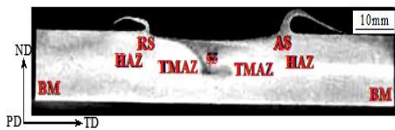
Figure 7 Cross section of FSP sample.
