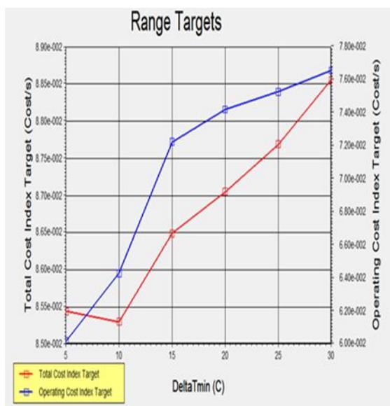
Figure 3  $\Delta T_{min}$  versus the total annualized cost.
