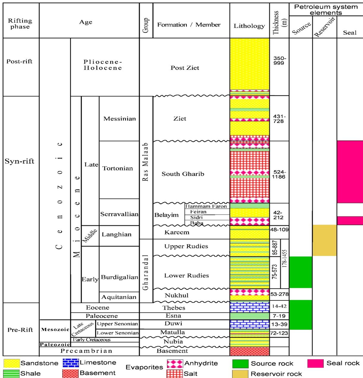
Figure 2 Lithostratigraphic column of the Garra area indicating elements of the petroleum system (Modified after Elmaadawy, 2020).
