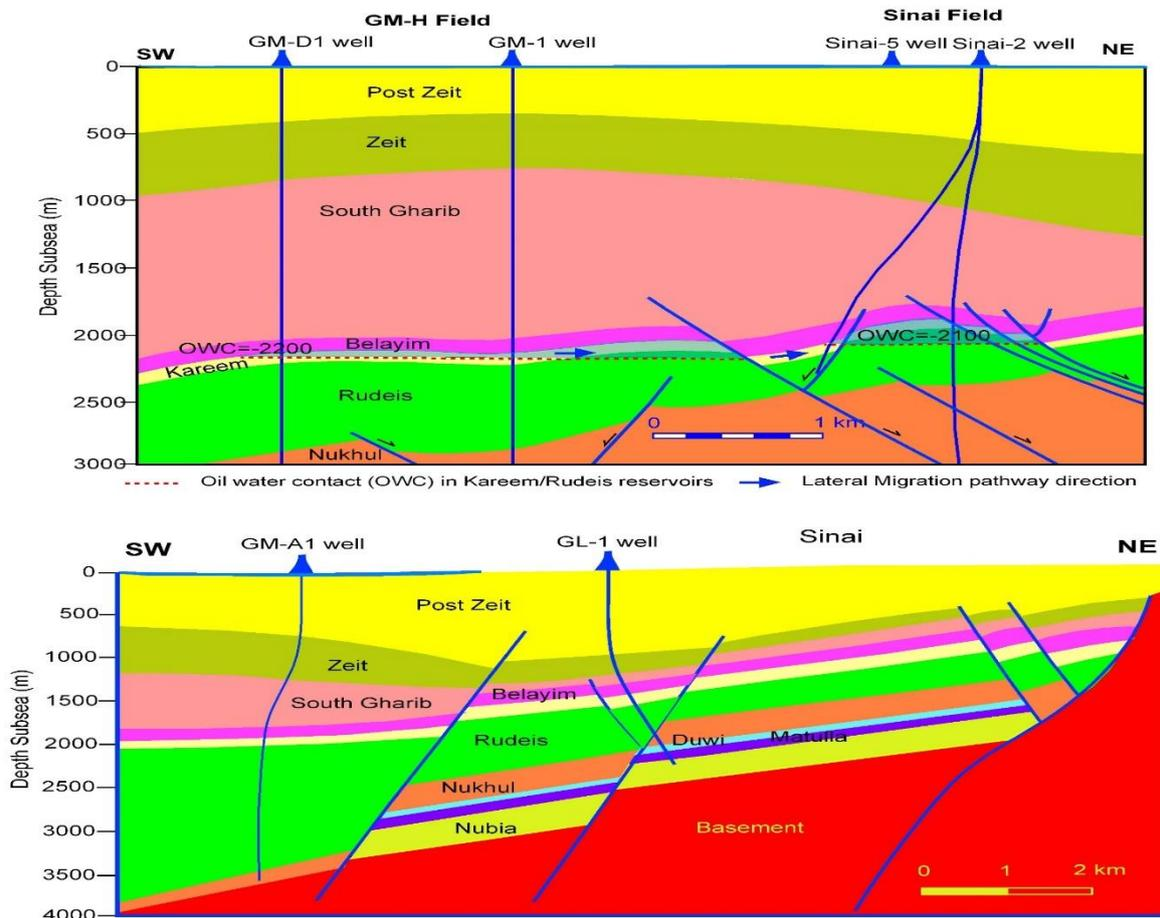
Figure 9 Geological cross-sections in Garra region indicate the direction of hydrocarbon migration to the northeast direction.
