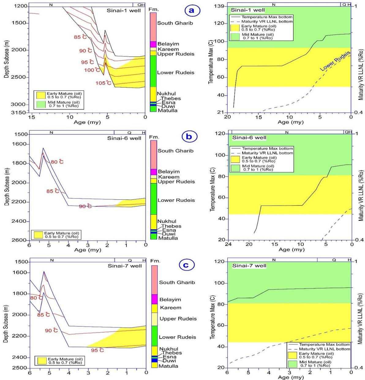
**Figure 6** The burial history and maturity models refer to stages of maturity, depth and time to maturity and distribution of temperature of the Lower Rudeis source rock in wells Sinai\_1 (a), Sinai\_6 (b) and Sinai\_7 (c).
