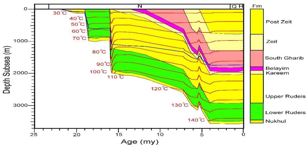
**Figure 3** The graph of the burial history showing the curves of tectonic subsidence of GM-A1 well.
