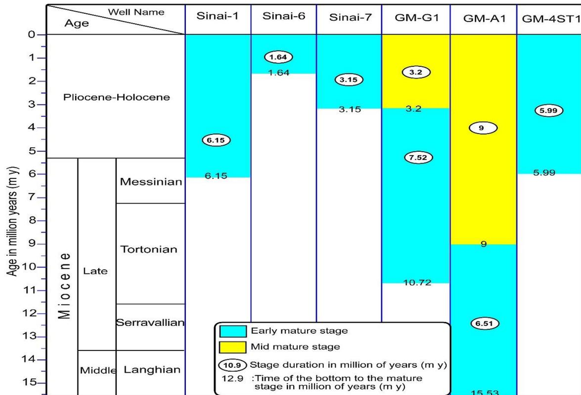
Figure 12 Graph indicating the early and mid-mature stage durations for the source rock of the Lower Rudeis
