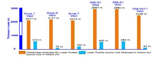
Figure 11 Thicknesses distribution of the Lower Rudeis source rock and overburden.
