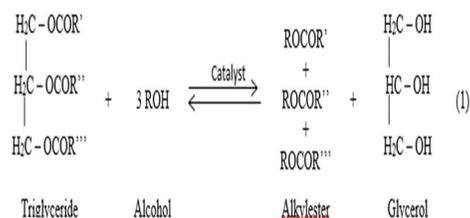
Transesterification process relies mainly on free fatty acid and water. Measurement of free fatty acid is a necessary before transesterification as it determines which type of catalyst will be more effective. Alkaline transesterification is most effective in feedstocks with free fatty acid (FFA) content less than 1%. KOH is the common catalyst used in alkaline transesterification and sulfuric acid is the common catalyst in acid transesterification<sup>[5, 12]</sup>.
