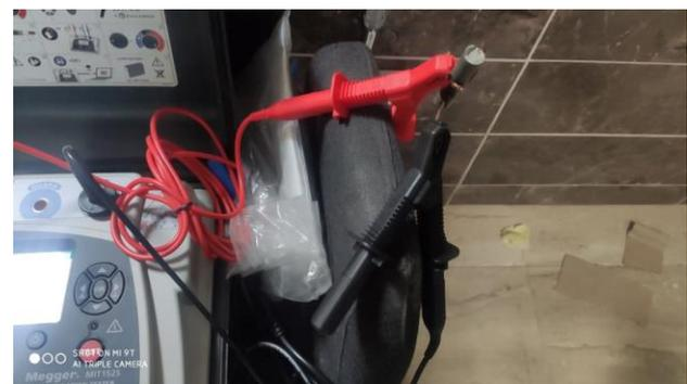
**Figure 1:** Measuring resistance values by insulation tester megger (MIT515) model.
