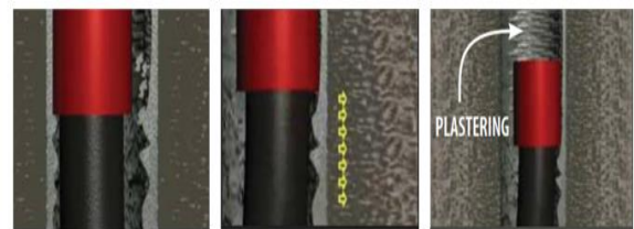
Fig. 1-a: Casing is forced against the bore wall as it advances into the borehole [5]. Fig. 1-b: As mud is smeared into the formation, filter cake builds up on the borehole wall [5]. Fig. 1-c: Filter cake and cuttings are plastered against the borehole wall, sealing porous formations [5].
