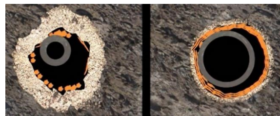
Figure 2 Drilling with conventional drill pipe (left) allows a larger annulus, while drilling with casing (right) minimizes annulus.
