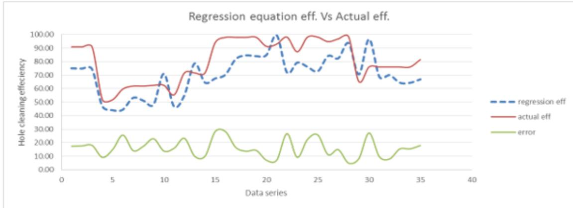
Figure 1 the regression equation results vs actual values of hole cleaning efficiency (20% of wells data)
