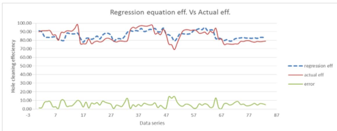
Figure 3 the regression equation results vs actual values of hole cleaning efficiency for the rest of data (80% of wells data)
