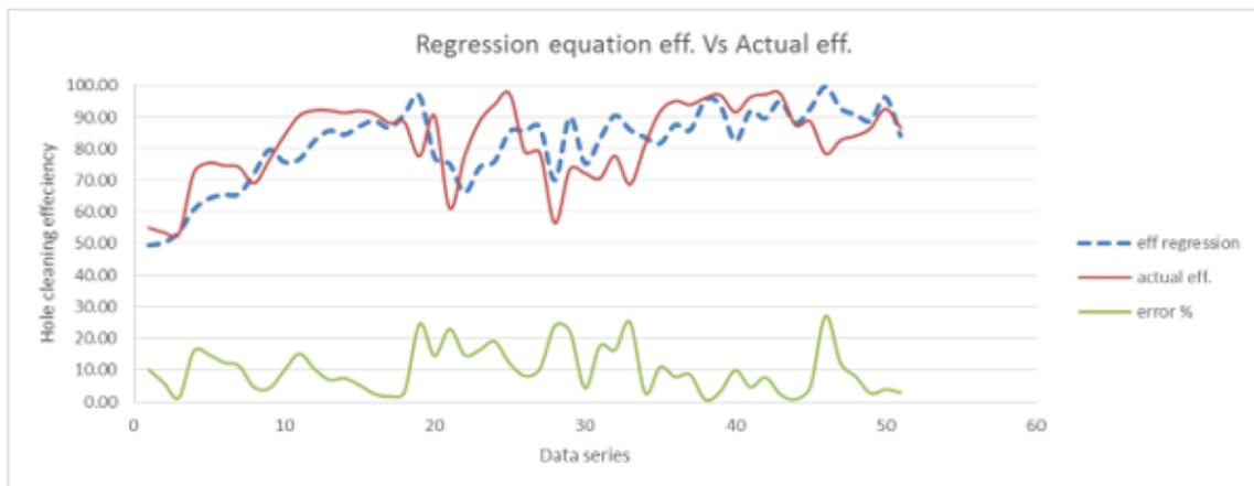
Figure 2 the regression equation results vs actual values of hole cleaning efficiency (40% of wells data)
