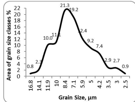
**Figure 10** Area percent of grain sizes against grain size classes for the fourth trial (at finishing temperature of 800°C).
