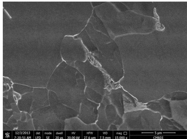
**Figure 7** SEM of lamellar pearlite morphology in after low finishing temperature (750°C); higher magnification from Figure 6.
