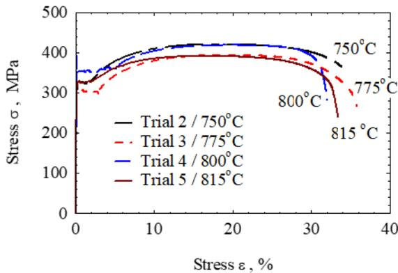
**Figure 9** Stress-strain curves for the trials group conducted at same strain and strain rate and at different finishing deformation temperatures.
