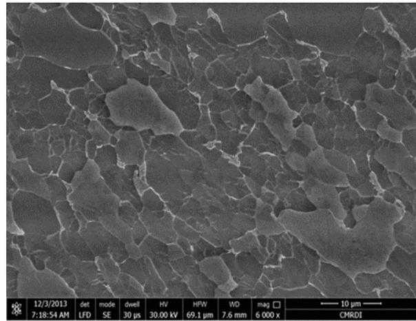
**Figure 6** SEM micrograph for steel after finishing temperature of 750°C.
