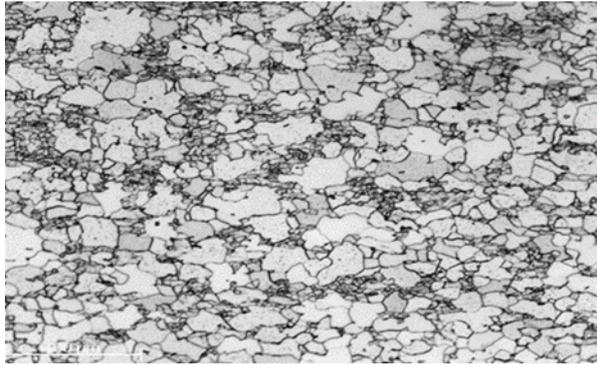
**Figure 3** Optical microstructure of the third trial, 775°C
