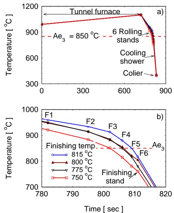
**Figure 1** (a) Temperature profile against rolling line and (b) closer description of the 6 rolling stands F1-F6 shown in (a).
