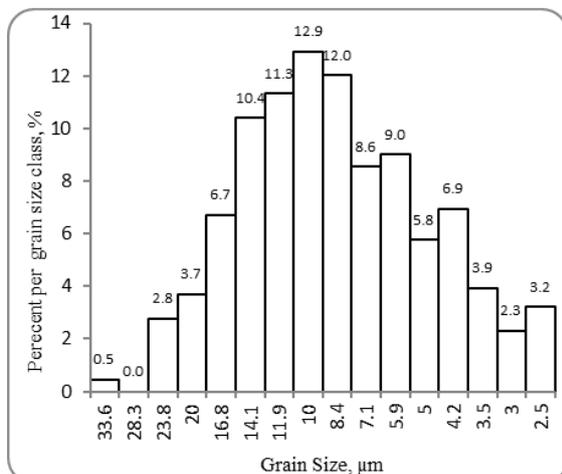
**Figure 5** The grain size distribution after a final deformation temperature of 775°C.
