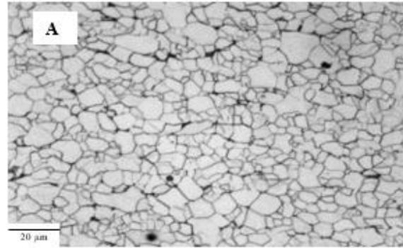
**Figure 4** Optical microstructure and SEM of the fourth trial, 800°C.
