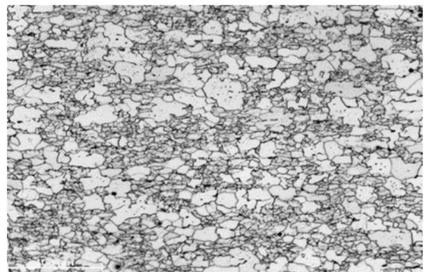
**Figure 2** Optical microstructure of second trial, 750°C
