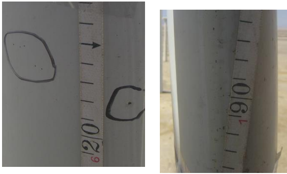
Figure 14 Examples of pin holes/coating pores.
