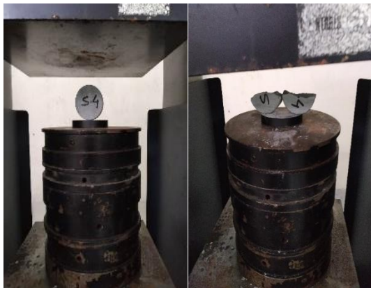
Figure 9 Position of disc specimen before and after to perform the Brazilian text.
