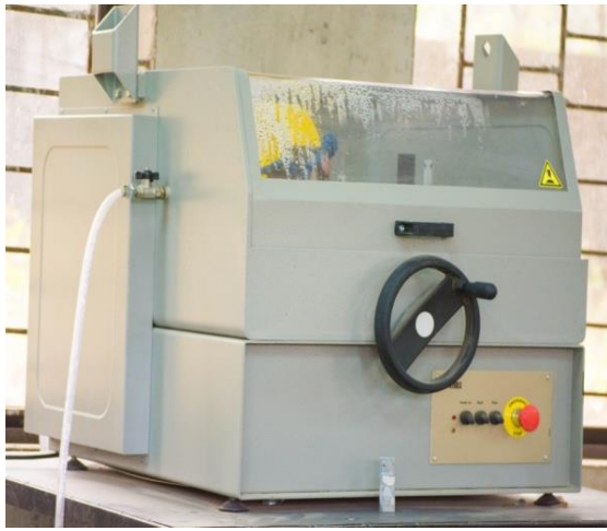
Figure 5 Core trimming machine to smoothen the rock specimen edge.
