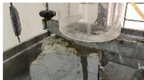
Figure 4 Core plugging machine to prepare the cylindrical core specimens.
