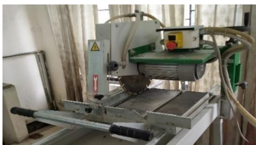
Figure 3 Diamond-saw cutter to cut the rock samples.
