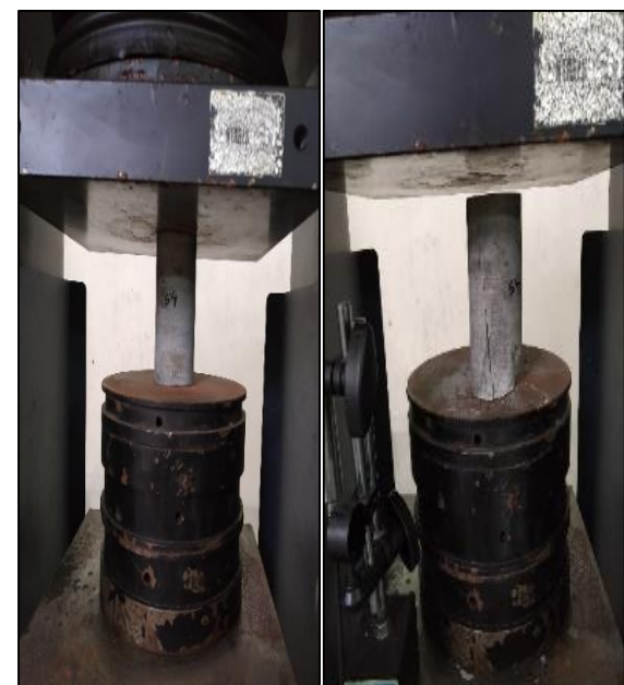
Figure 8 Cylindrical specimen before and after the uniaxial compression test
