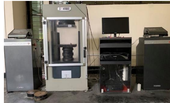
Figure 7 Compression testing machine for rock strength measurement.
