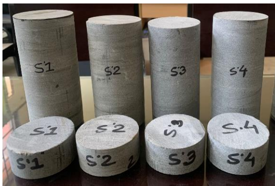
Figure 6 Cylindrical and disc specimens prepared for rock strength tests.
