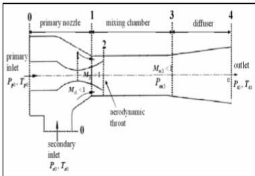
Figure 4. schematic of gas ejector model.
