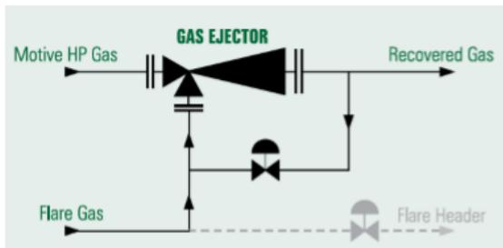
Figure 1. Flare gas recovery unit Using gas ejector.
