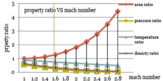
Figure 6. plot Mach number vs. & property ratio.
