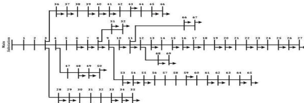
Figure 2 Single line diagram of IEEE 69 bus network
