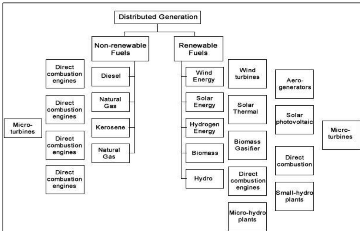
**Figure 1** Distribution Generation technologie
