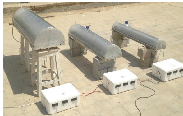
Figure 3 Experimental set-up of the half-TSS model with variable tray dimensions
